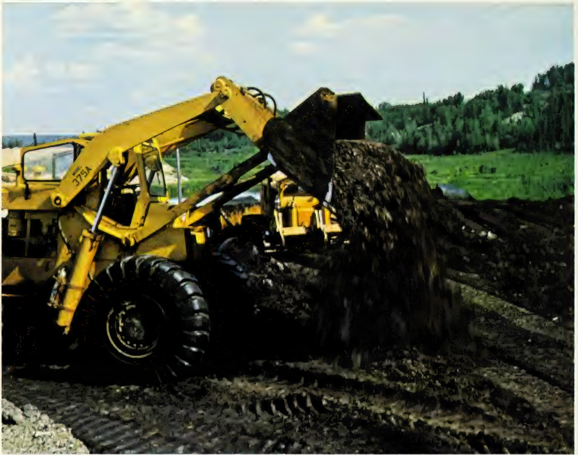
It is estimated that 300 billion barrels of marketable crude oil are contained in the Athabasca oil sands. Found near the surface, the oil-bearing sands can be strip-mined, like a mineral.
